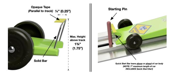
• Cars with Indented Noses like the one pictured below are prohibited <u>unless</u> the Car is fitted with a properly installed "Quick Start" front end, as described above. An indented nose causes the Car to stage further down the track against the starting pin, which unfairly shortens the Car's course relative to the other Cars in the race.
