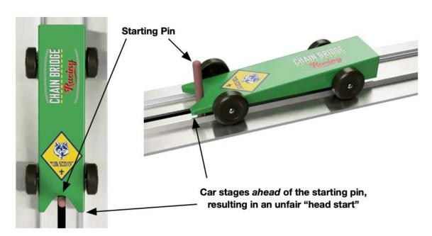
• Cars with Sharp or Very Narrow Pointed Noses like the one pictured below are *prohibited*. Cars with this shape may not properly rest against the pin at the starting gate and can lead to false starts.
