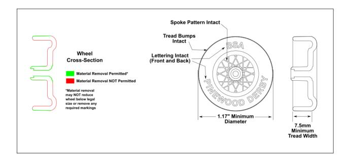
Bearings and bushings are not permitted to be used inside the wheels. You are not permitted to fill the bores with foreign material and re-bore. The inner hubs of the wheels must be able to make contact with the sides of the car.
